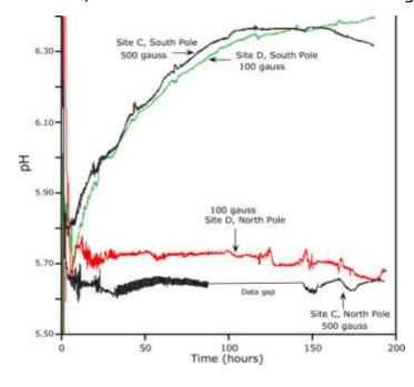
Figure 2. pH changes with time for pure water for both N-pole up and S-pole up axially aligned DC magnetic fields at 100 and 500 gauss.
