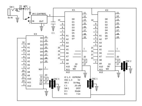
Figure 1. Circuit diagram for the electronic devices used as host devices for our intention imprinting.
